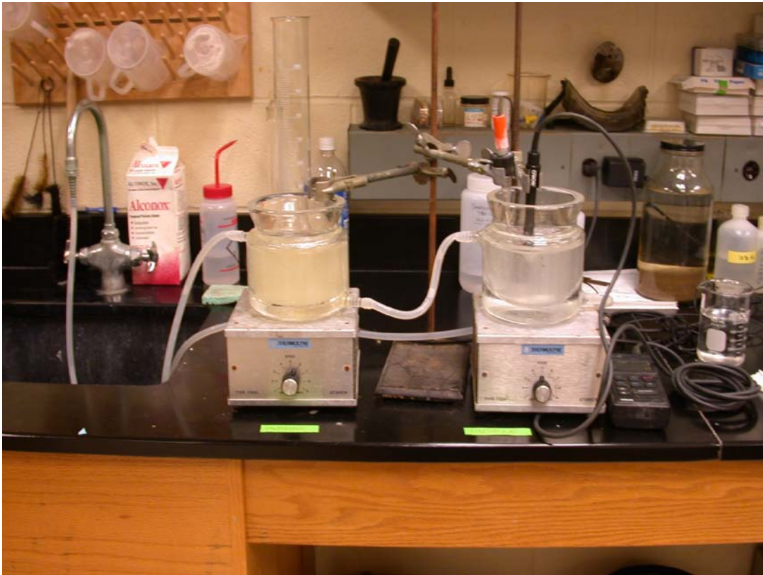
Figure 6. Experimental set-up for batch experiments. pH and conductivity continuously monitored. Flat vessel on the left and round vessel on the right.
